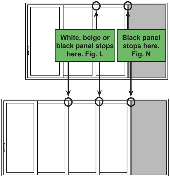
21. In the hardware box you will find white, beige or black Panel Stops, depending on the color of the door. (Fig. K). These will be mounted on the top of the 2nd and/or 3rd intermediate panels. (Fig. L)
