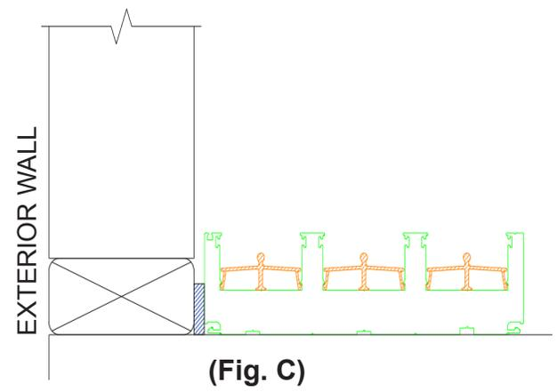
3 track screw placement. Do not pre-drill 3/8 hole on the die lines.
